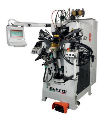
New generation of heel seat and side lasting machine, for a constant precision and rapidity of execution, with hydraulic functioning with some pneumatic movements, with on screen programming of the insole profile, from the heel to the ball and simultaneous positioning of the side lasting.
